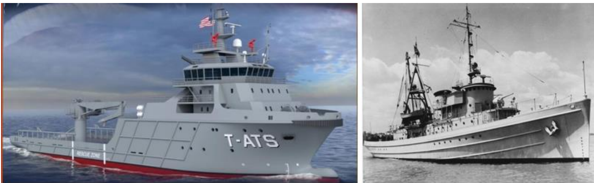
An artist rendering (left) of the future towing, salvage, and rescue ship Cherokee Nation being built to replace the Powhatan-class fleet ocean tugs (T-ATF 166) on the right
